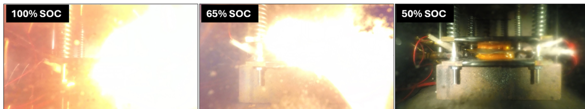
Extended Data Fig. 2 | Internal short circuiting of liquid-electrolyte graphite/NCM811 LiBs at various state of charge (SOC). a , Temporal variations of voltage, shorting current, shorting resistance and internal temperature at 100%, 65% and 50% SOC, respectively. b , Photographic images of LiB cells after ISC. The 100%
